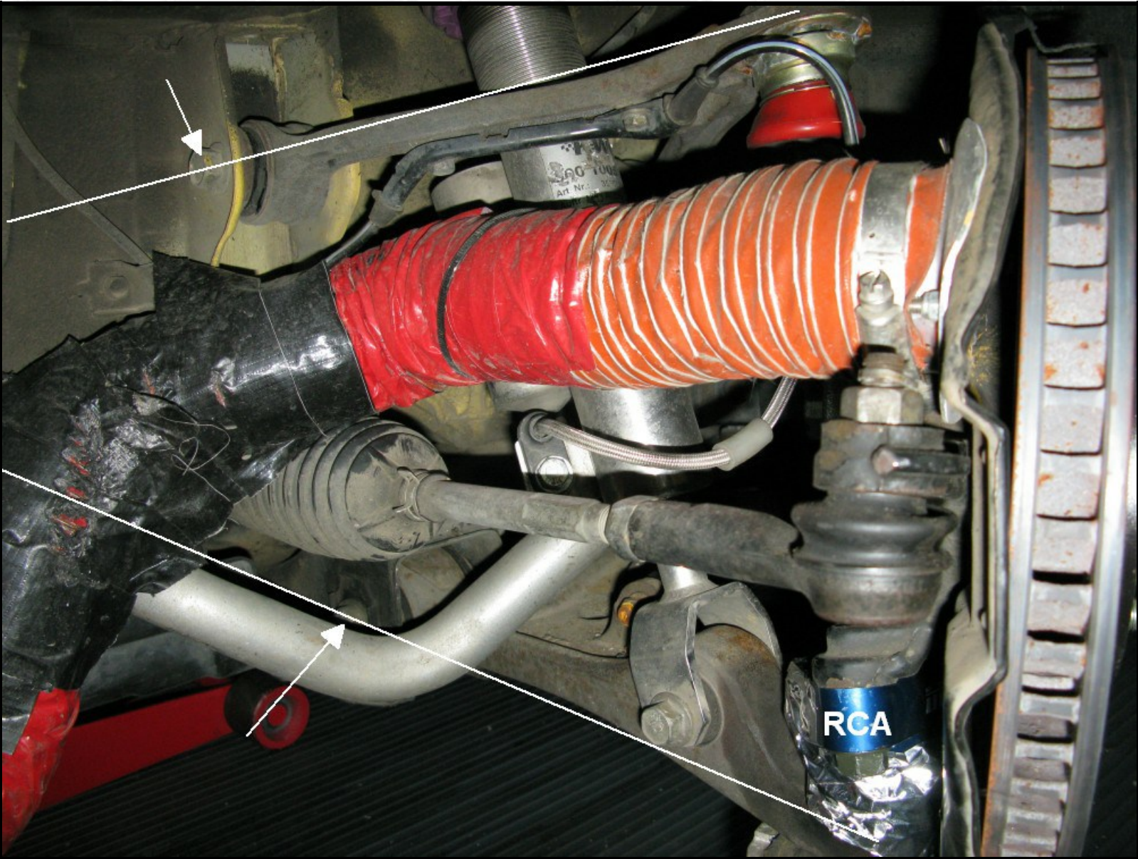
1 inch Lowered with Roll Center Adjusters
