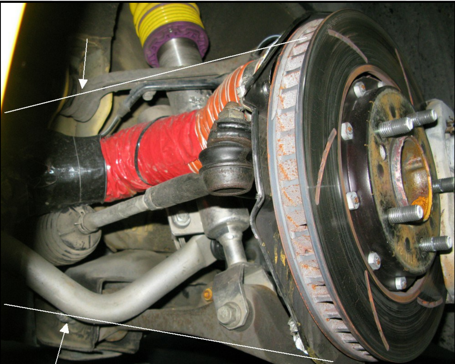
1 inch Lowered S2000's Front Control Arm Angles Before Roll Center Adjusters
