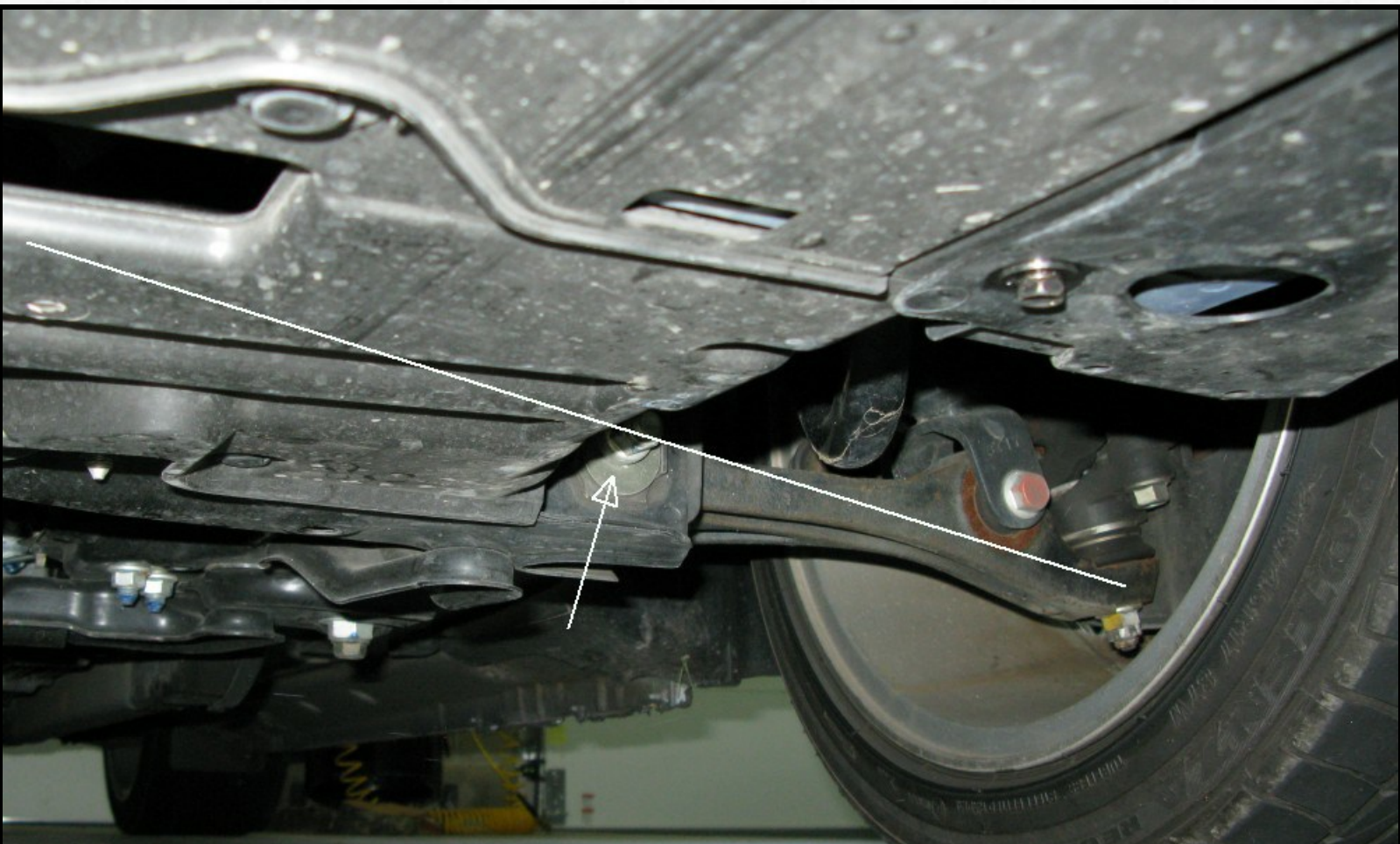
Stock AP2 S2000's Front Lower Control Arm Angle
