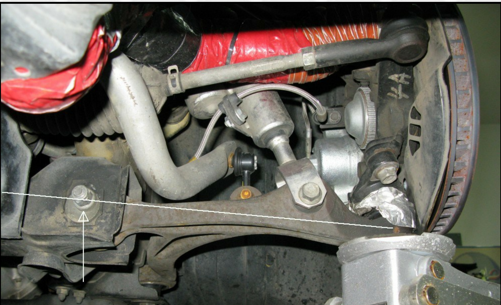
1 inch Lowered S2000's Front Lower Control Arm
