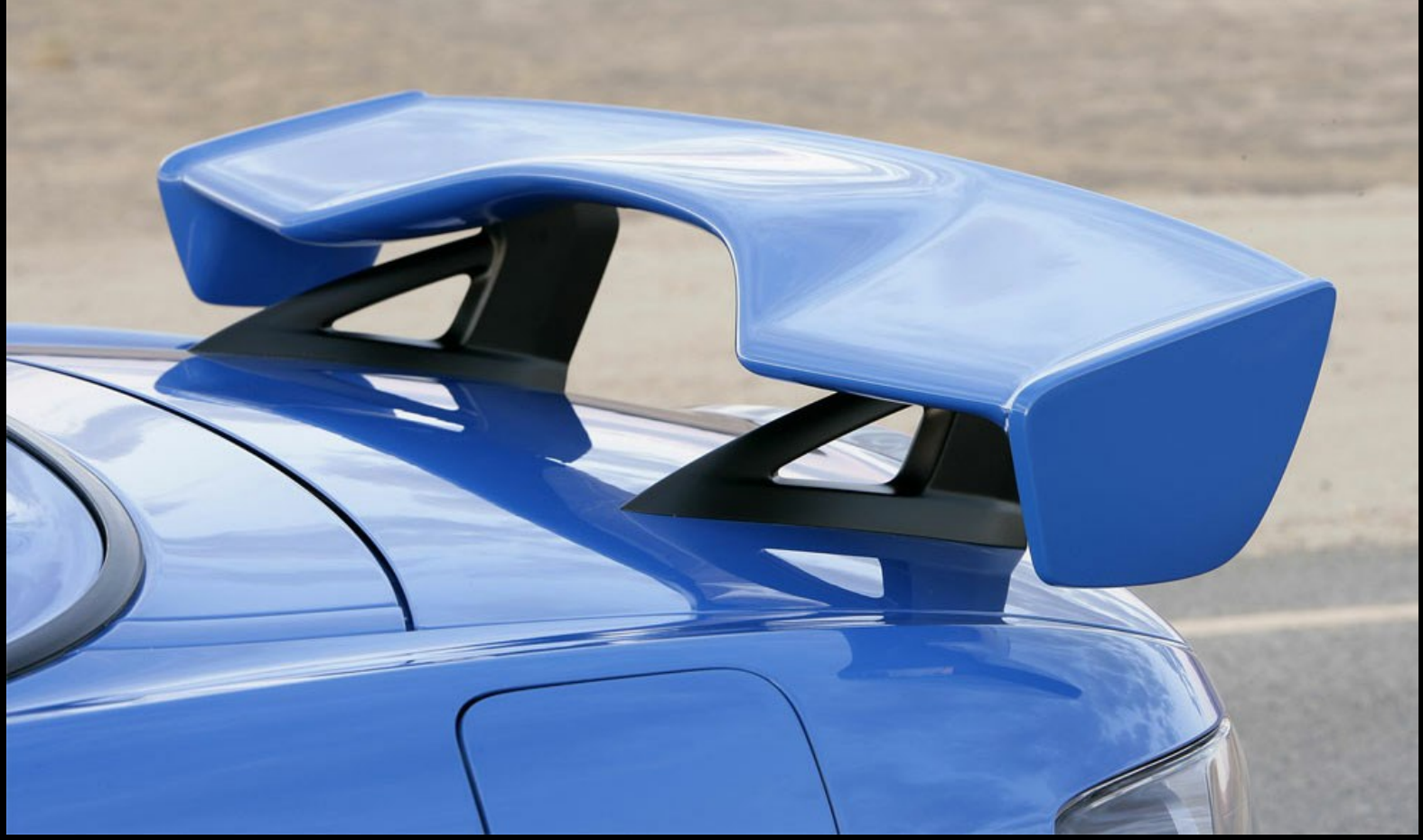
The CR wing is a medium mount, 3D profile wing with good size end plates. It has proven to be an effective track wing for racing and time trial.
