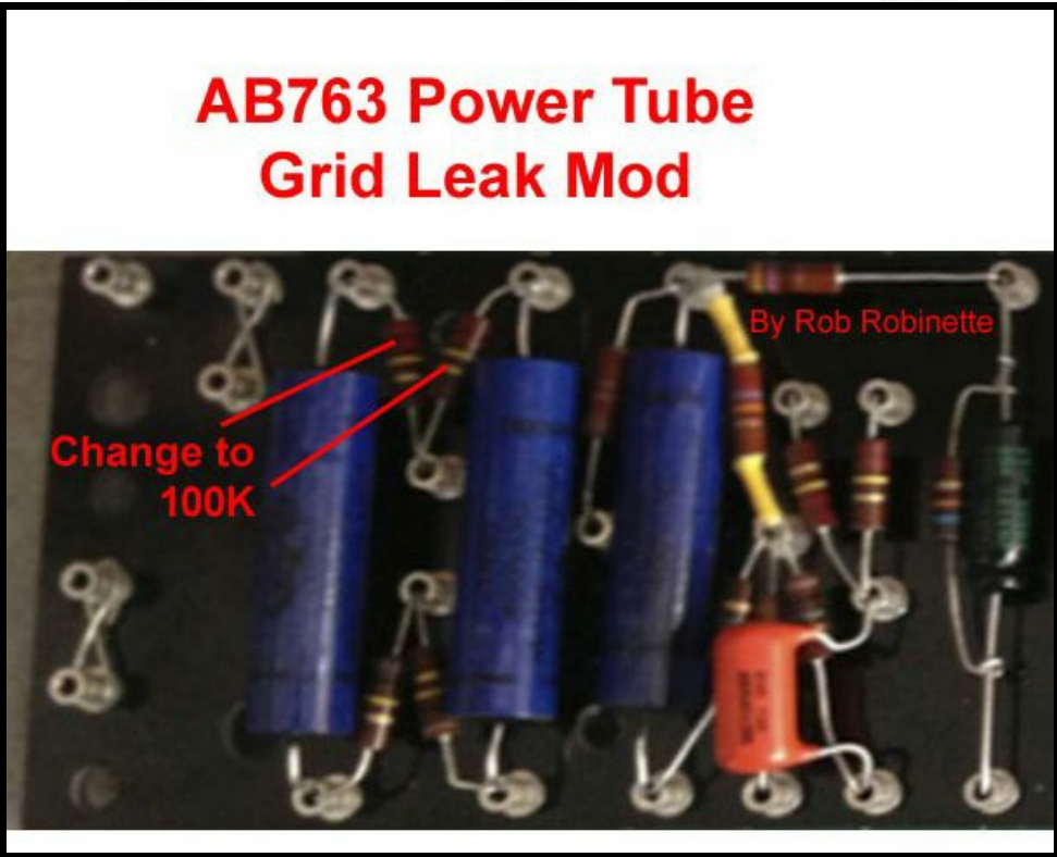
The 220k 1/2 watt power tube grid leak resistors are on the far left end of the circuit board.
