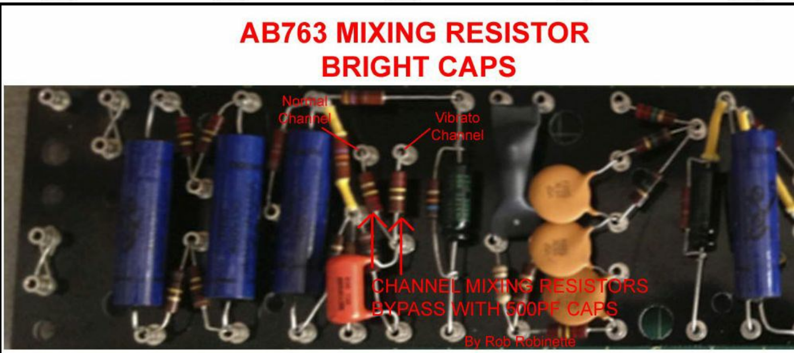
The 220k Channel Mixing resistor on the left is the Normal Channel's, the Vibrato Channel's resistor is on the right. Original photo by John Chabalko.
