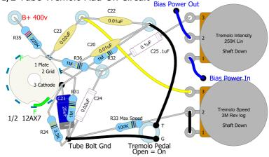
Circuit based on AA1164 Blackface Princeton Reverb tremolo. Layout by Rob Robinette Circuit is a tube oscillator attached to power tube fixed bias power supply. Circuit is inserted between power tube fixed bias supply and grid resistors. 'Bias Power Out' connects to the junction of the power tube grid resistors. 'Bias Power In' connects to the bias power supply output. See AA1164 Schematic for details.
