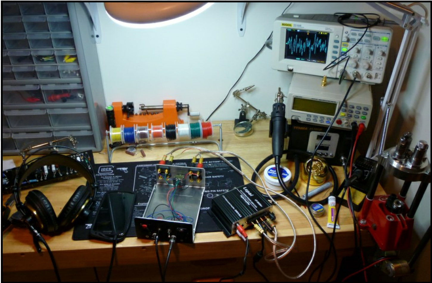
Testing 'Amp Mode Switch' with single-ended headphones and balanced output amplifier.
